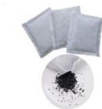
As shown in the image small pouches from bamboo carbon were made. These pouches are capable of removing odor and moisture from the container in which they are kept.
