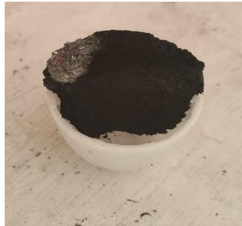
Carbon Briquettes of the size of a Biscuit were prepared from the bamboo Carbon. As shown in the second image the briquette burnt continuously without any smoke and the small briquette was able to raise the temperature of the cup to 320 °C.
